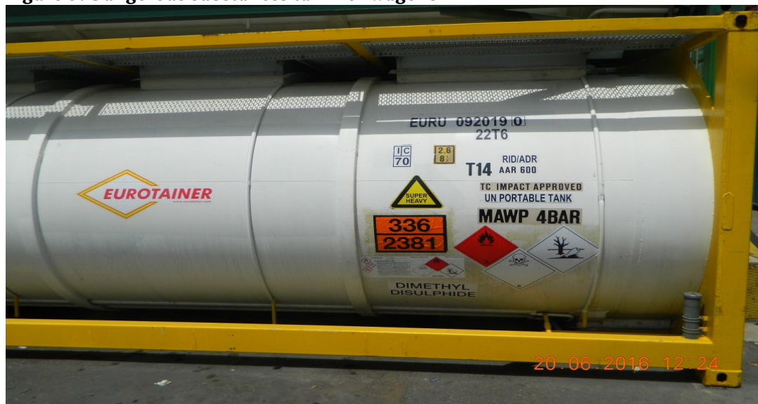
Figure 5: Dangerous substances tank for wagons
